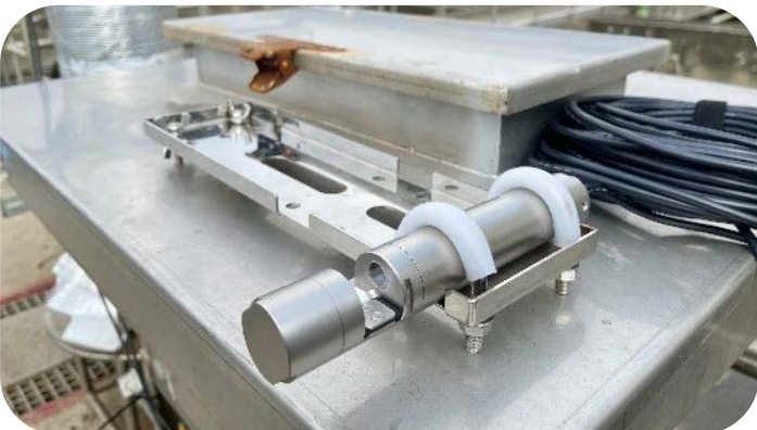
Example of Actual Installation of Turbidity Sensor at Customer's End
